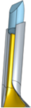
Figure 1: steering head on curved tape spring needle body with inner tape spring as control transmission.
